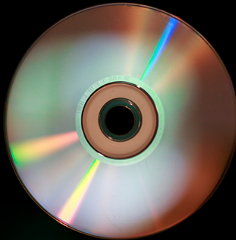
Figure 27.1 The colors reflected by this compact disc vary with angle and are not caused by pigments. Colors such as these are direct evidence of the wave character of light. (credit: Reggie Mathalone)
